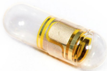
Figure 1a. ID-Capsule: A Digital Pill Consisting of a Pharmaceutical-Grade Capsule Shell with an Embedded Ingestible Sensor
