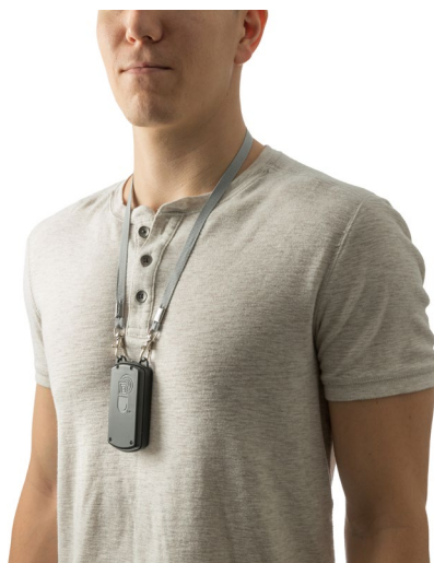
Figure 1b. Reader: A Wearable Device that Detects Messages Transmitted from the Ingested Sensor and Forwards them to the Patient App and Clinician Dashboard
